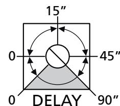
**DELAY:** time delay between the two gate leaves (0 - 90 seconds).
